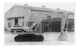
This machine is equipped with a 3066 direct injection turbocharged engine and other specifically developed systems and components such as electronic power unit control system, work mode choice system, two-speed travel motor, etc. The machine is designed primarily for excavating and loading material.
