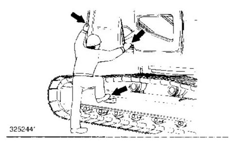
\* Face the machine when mounting and dismounting.
