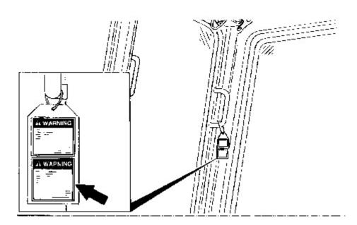
Located in the cab on machines equipped with air conditioning systems containing R-12 air conditioner refrigerant (if equipped).
