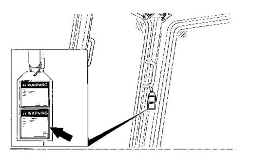
Located in the cab on machines equipped with air conditioning systems containing R-12 air conditioner refrigerant (if equipped).
