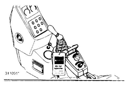
Attach a Do Not Operate, SEHS7332, or similar warning tag to start switch or controls before servicing or repairing the machine. This tag is available from your Caterpillar dealer.
