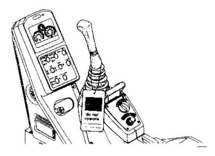
Attach a DO NOT OPERATE, SEHS7332, or similar warning tag to start switch or controls before servicing or repairing the machine. This tag is available from your Caterpillar dealer.
