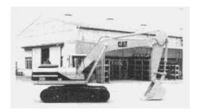
This machine is equipped with a direct injection 3116 turbocharged engine and other specifically developed systems and components such as electronic power unit control system, work mode choice system, two-speed travel motor, etc. The machine is designed primarily for excavating and loading material.
