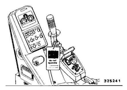
Attach a DO NOT OPERATE, SEHS7332, or similar warning tag to start switch or controls before servicing or repairing the machine. This tag is available from your Caterpillar dealer.
