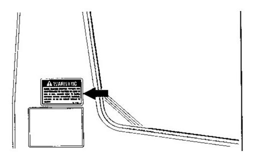
Located on the outside surface of the cab, if the machine is 2-way valve equipped.
