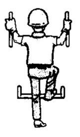
\* Mount and dismount the machine only where steps and/or handholds are provided.
