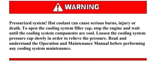
Refer to Operation and Maintenance Manual, "Cooling System Coolant Level - Check" for further information.
