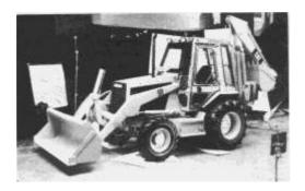
Park on a level surface if possible. If necessary to park on a grade, block the machine.Apply the service brakes to stop the machine. Engage the parking brake.Shift the transmission control levers to NEUTRAL. Apply the neutral lock.Lower the loader bucket to the ground and apply slight down pressure.Put the backhoe in the "transport position". Install the swing lock pin in backhoe.Stop the engine.
