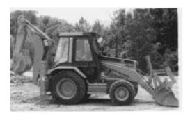
Park on a level surface. If necessary to park on a grade, block the machine.
