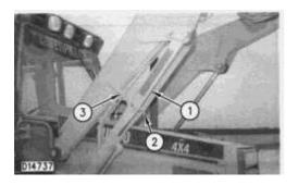
When performing any work underneath a raised loader lift arm, the loader lift arm brace (1) must be in place as shown.
