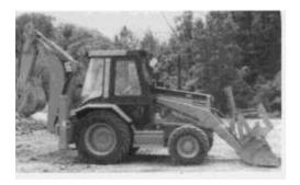
This machine is equipped with a 3054 diesel engine. It has a four-speed transmission and is designed primarily for moving material.
