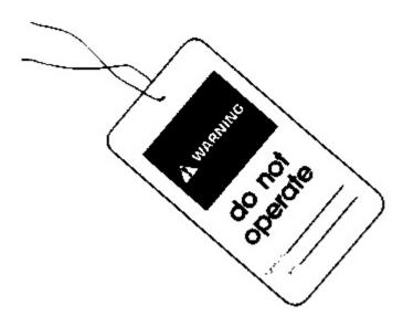
Attach a "DO NOT OPERATE" or similar warning tag to start switch or controls before servicing or repairing the machine. These tags, Form SEHS7332, are available from your Caterpillar dealer.
