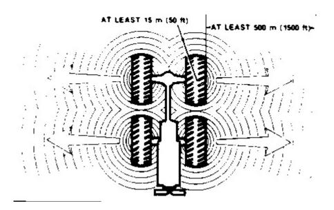
Do not approach a warm tire closer than the outside of the area represented by the shaded area in the above drawing.
