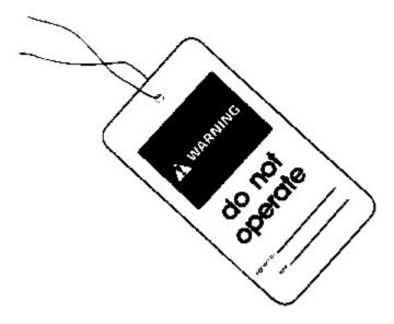
Attach a Do Not Operate, SEHS7332, or similar warning tag to start switch or controls before servicing or repairing the machine. This tag is available from your Caterpillar dealer.
