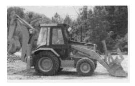
This machine is equipped with a 3054 diesel engine. It has a four-speed transmission and is designed primarily for moving material.
