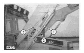
When performing any work underneath a raised loader lift arm, the loader lift arm brace (1) must be in place as shown.
