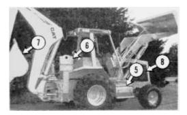
Battery compartment (5), stabilizer (6), backhoe bucket (7) and radiator (8).
