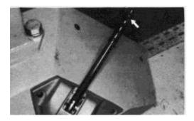
Pull the parking brake lever up to activate indicator and engage parking brake.
