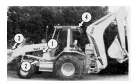
Engine (1), fuel tank (2), loader bucket (3), cab or canopy (4).
