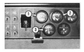
**Engine Coolant (1)** - Indicates the coolant temperature. If the temperature is excessive, 107°C (225°F) or above, stop the machine. Investigate the cause and correct the problem before operating again.
