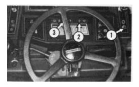
**Panel Test Switch (1)** - With the engine stopped and the ignition on, move test switch UP. Indicator lights (2) and (3) should come on until the switch is released. Release the switch. It will return to the OFF position.
