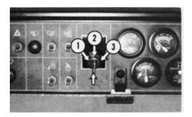
**OFF (1)** - Turn the key to OFF to stop the engine. To insert or remove the key, the key must be in this position. Also, to keep the fault alarm from sounding.
