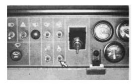
Starting Aid - Move the switch and release to inject a metered amount of ether.
