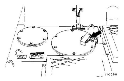
Remove the hydraulic tank filler cap only after the engine has been stopped and the filler cap is cool enough to remove with your bare hand.
