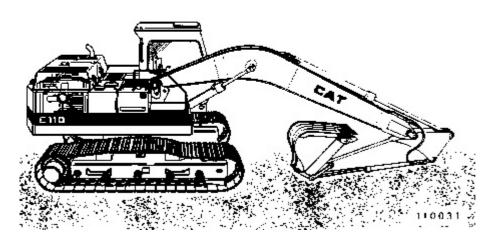
Park on a level surface. If necessary to park on a grade, block the machine. Place the implements in the servicing position. (See illustration above.)
