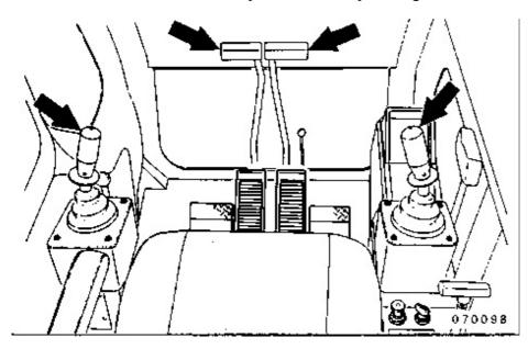
**2.** Release the internal pressure from the hydraulic system by manipulating the travel levers back and forth, and the R.H. and L.H. control levers in all directions (back and forth, left and right).
