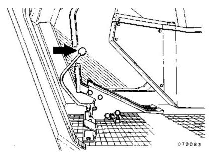
Move the travel lock lever to the locked position.
