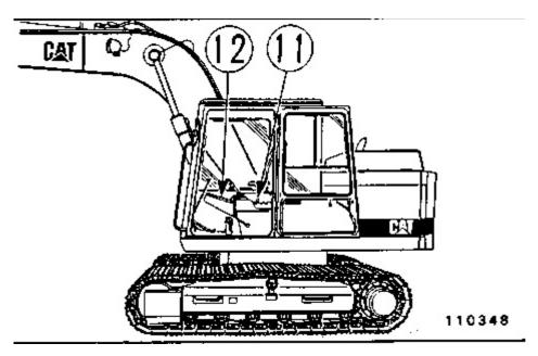
Start switch key (11) and electronic monitoring system (12).
