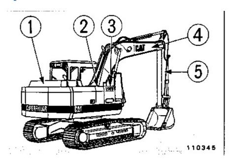
Engine (1), hydraulic tank (2), fuel tank (3), boom (4), and stick (5).
