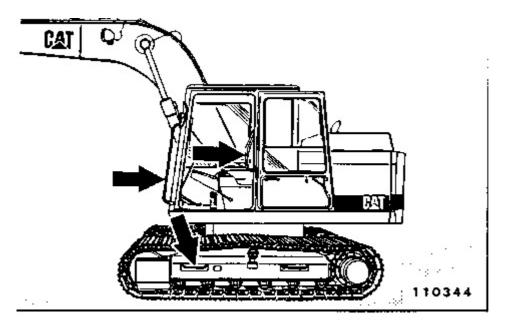
Mount and dismount the machine only where steps and/or handholds are provided.
