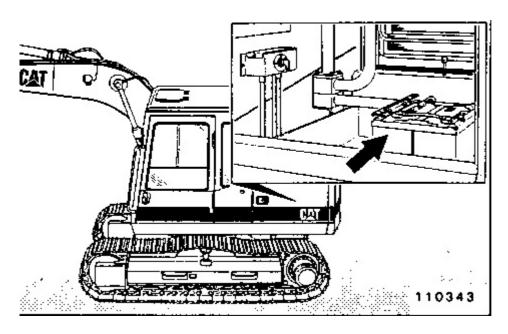
Batteries give off flammable fumes which can explode. Do not smoke when observing the battery electrolyte levels. Electrolyte is an acid and can cause personal injury if it contacts skin or eyes.
