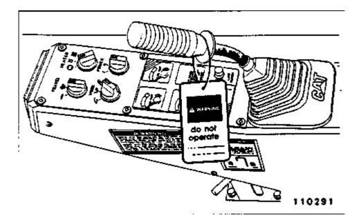
Attach a "DO NOT OPERATE" or similar warning tag to start switch or controls before servicing or repairing the machine. These tags, Form SEHS 7332 are available from your Caterpillar dealer.
