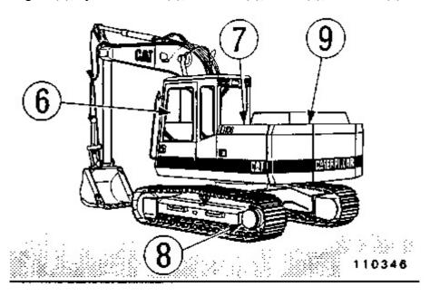
Operator's compartment (6), radiator (7), final drive (8), and counterweight (9).
