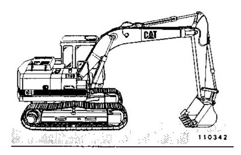
This machine is equipped with a direct injection 3114T turbocharged engine and other specifically developed systems and components such as electronic power unit control system, work mode choice system, 2 - speed travel motor, etc.
