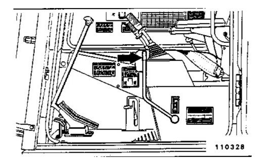
Move the hydraulic activation control lever to the locked position.
