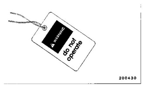
Do not start the engine or move any of the controls if there is a "DO NOT OPERATE" or similar warning tag attached to the start switch or controls.
