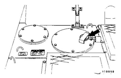
Remove the hydraulic tank filler cap only after the engine has been stopped and the filler cap is cool enough to remove with your bare hand.
