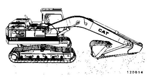
Park on a level surface. If necessary to park on a grade, block the machine.
