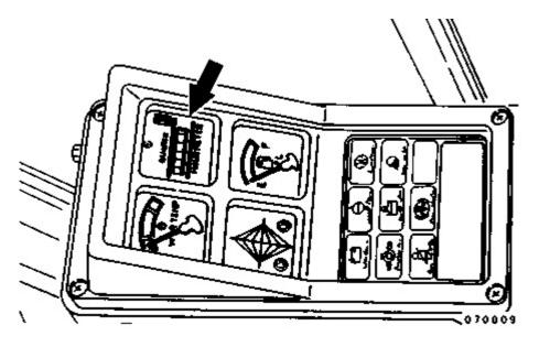
Use the service hour meter to determine servicing intervals. Calendar intervals shown (daily, weekly, monthly, etc.) may be used instead of service hour meter intervals if they provide more convenient servicing schedules and approximate the indicated service hour meter reading. Recommended service should always be performed at the interval that occurs first.
