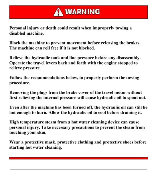
To tow the machine, both final drives must be disengaged.
