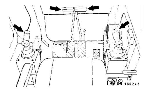
**2.** Operate the travel and control levers to relieve hydraulic line pressure.
