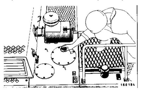
**3.** Loosen the pressure cap to relieve the hydraulic tank pressure.
