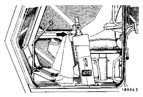
Move the hydraulic activation control lever to the locked position.
