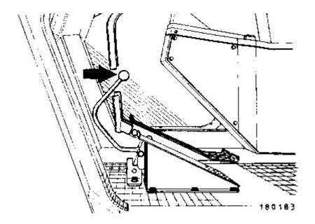
Move the travel lock lever to the locked position.
