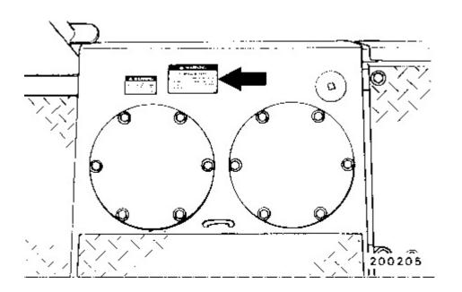
Located on the hydraulic tank.
