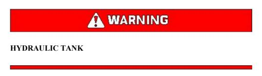
Relieve tank pressure with engine off by removing cap slowly to prevent burns from hot oil.
