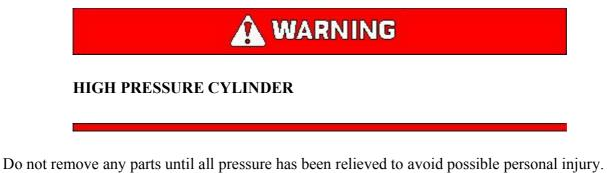
Do not remove any parts until all pressure has been relieved to avoid possible personal injury. Relieve pressure by opening relief valve 1 turn maximum.
