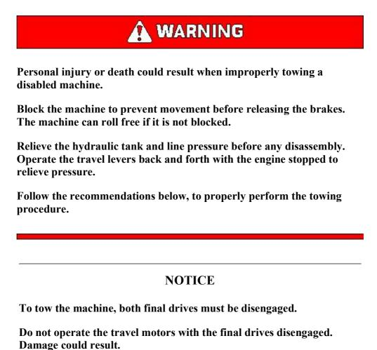
These towing instructions are for moving a disabled machine a short distance, only a few feet at low speed, no faster than 2 km/h (1.2 mph), to a convenient location for repair. These instructions are for emergencies only. Always haul the machine if long distance moving is required.
