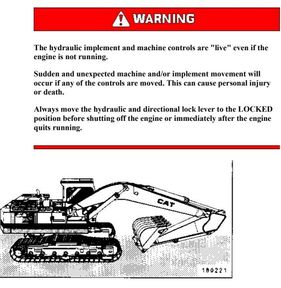
Park on a level surface. If necessary to park on a grade, block the machine.
