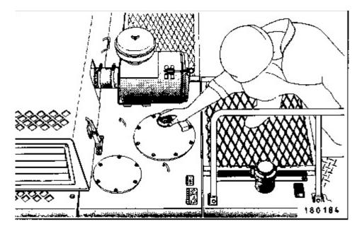
**3.** Loosen the pressure cap to relieve the hydraulic tank pressure.
