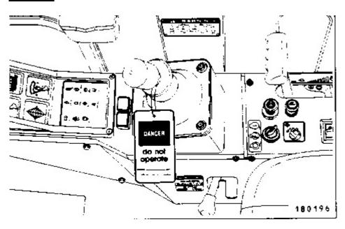
Attach a "DO NOT OPERATE" or similar warning tag to start switch or controls before servicing or repairing the machine. These tags, Form SEHS7332 are available from your Caterpillar dealer.
