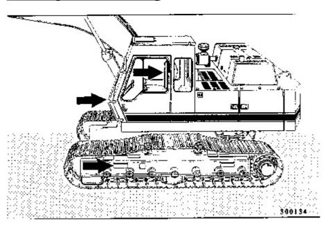
Mount and dismount the machine only where steps and/or handholds are provided.
