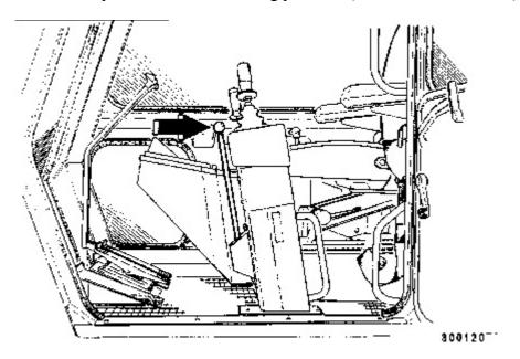
Move the hydraulic activation control lever to the locked position.
