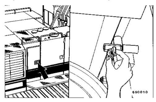
**3.** Open the valve of the hydraulic tank to relieve the pressure.
