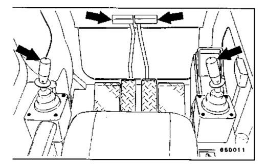
**4.** With engine stopped relieve the internal pressure from the hydraulic system by manipulating the travel levers back and forth, and the R.H. and L.H. control levers in all directions (back and forth, left and right).
