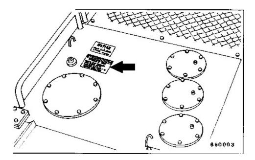
Located on the hydraulic tank.
