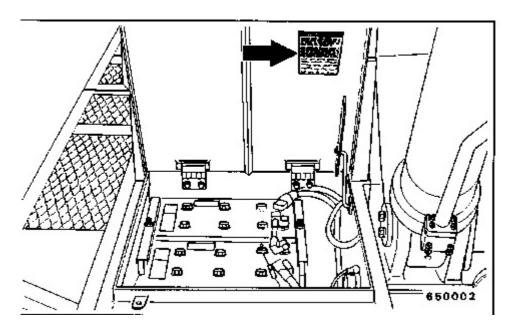
Located on the battery compartment cover.
