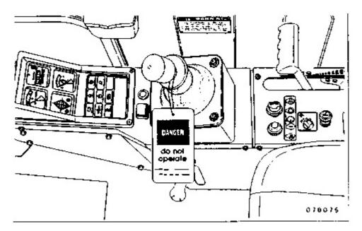
Attach a "DO NOT OPERATE" or similar warning tag to start switch or controls before servicing or repairing the machine. These tags, Form SEHS7332 are available from your Caterpillar dealer.
