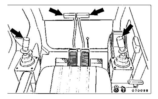
**2.** Operate the travel and control levers to relieve hydraulic line pressure.
