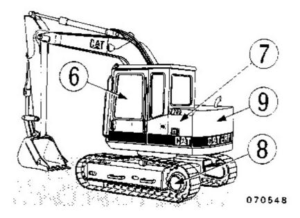
Operator's compartment (6), radiator (7), final drive (8) and counterweight (9).
