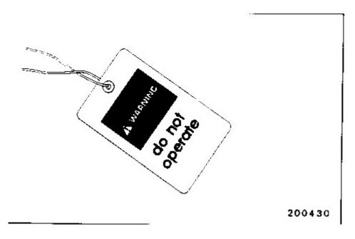
Do not start the engine or move any of the controls if there is a "DO NOT OPERATE" or similar warning tag attached to the start switch or controls.
