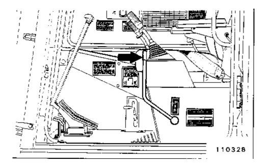
Move the hydraulic activation control lever to the locked position.
