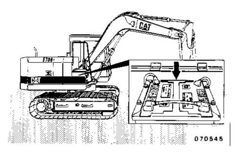
Batteries give off flammable fumes which can explode. Do not smoke when observing the battery electrolyte levels. Electrolyte is an acid and can cause personal injury if it contacts skin or eyes.
