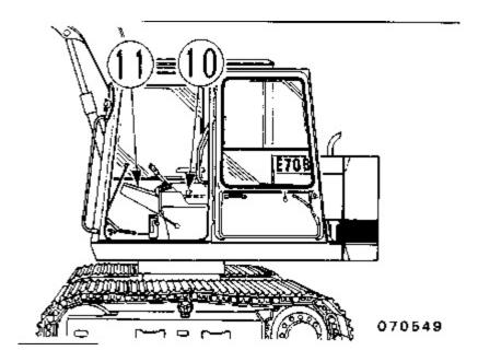
Start switch key (10) and electronic monitoring system (11).
