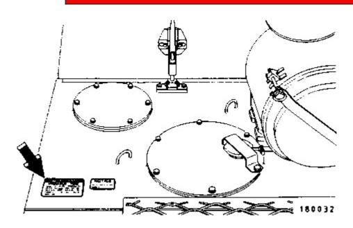
Located on the hydraulic tank.
