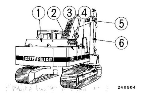
Engine (1), radiator (2), hydraulic tank (3), fuel tank (4), boom (5), and stick (6).
