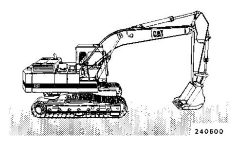
This machine is equipped with a direct injection 3116T turbocharged engine and other specifically developed systems and components such as electronic power unit control system, work mode choice system, etc.
