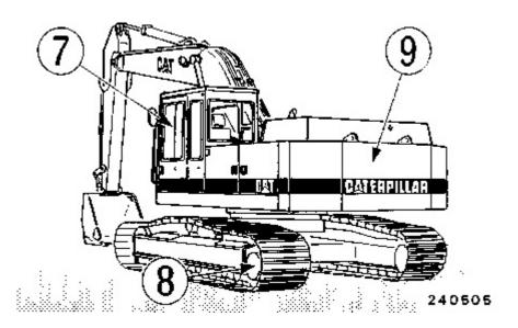
Operator's compartment (7), final drive (8), and counterweight (9).
