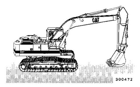
This machine is equipped with a direct injection 3306T turbocharged engine and other specifically developed systems and components such as electronic power unit control system, work mode choice system, 2 - speed travel motor, etc.
