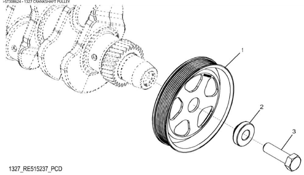
John Deere > Construction And Forestry > BACKHOE, LOADER > 310J - BACKHOE, LOADER > 310J Backhoe Loader > 04A ENGINE 4045HL287-SE503032 > 0400A ENGINE 4045HL287-SE503032 4045HL287 > ST308624 - 1327 CRANKSHAFT PULLEY
