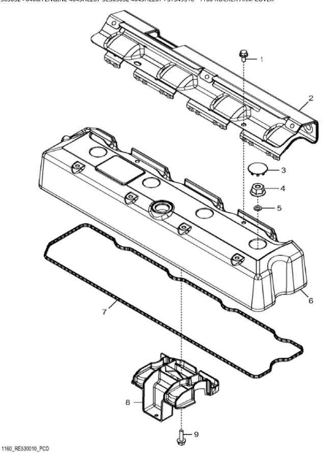
John Deere > Construction And Forestry > BACKHOE, LOADER > 310J - BACKHOE, LOADER > 310J Backhoe Loader > 04A ENGINE 4045HL287-SE503032 > 0400A ENGINE 4045HL287-SE503032 4045HL287 > ST349518 - 1160 ROCKER ARM COVER
