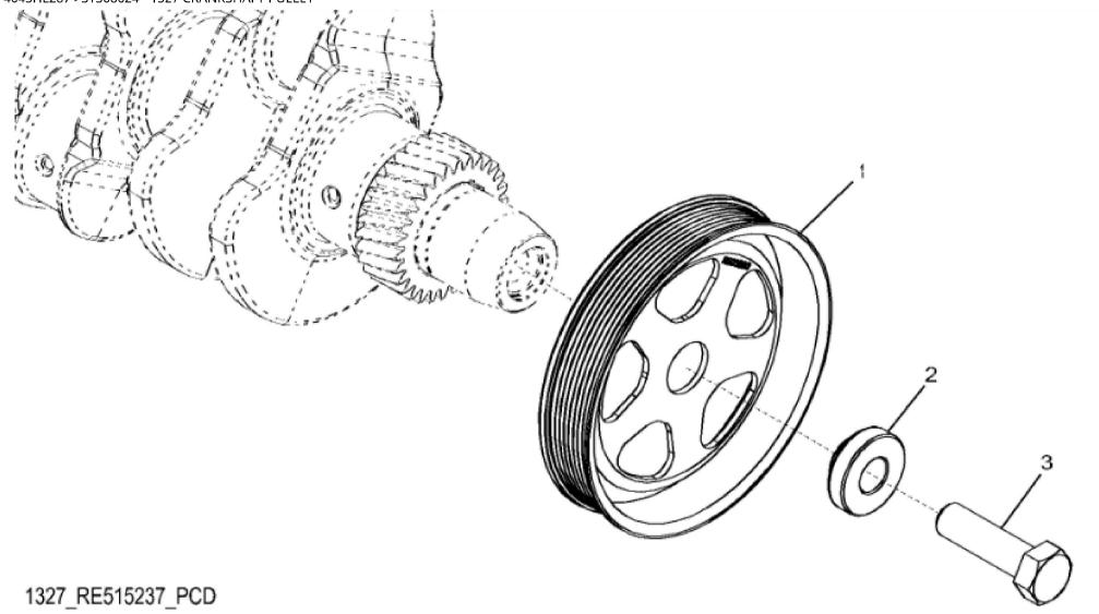
John Deere > Construction And Forestry >BACKHOE, LOADER >310TJ - BACKHOE, LOADER >310SJ TMC Backhoe Loader >04A ENGINE 4045HL287-SE503032 >0400A ENGINE 4045HL287-SE503032 4045HL287 >ST308624 - 1327 CRANKSHAFT PULLEY
