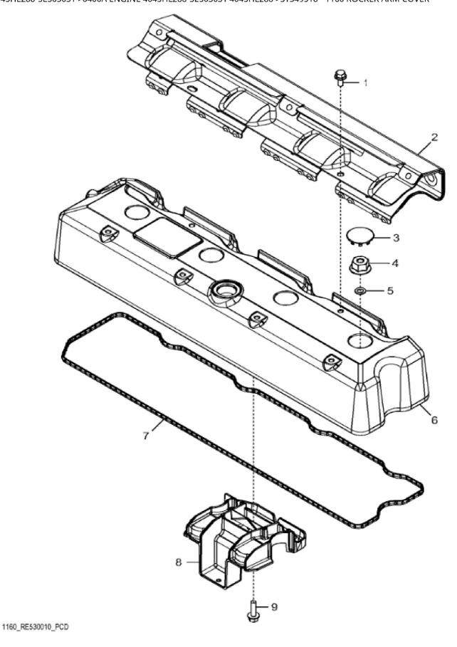
John Deere > Construction And Forestry >BACKHOE, LOADER >410J TMC - BACKHOE, LOADER >410J TMC Backhoe Loader >04A ENGINE 4045HL288-SE503031 >0400A ENGINE 4045HL288-SE503031 4045HL288 >ST349518 - 1160 ROCKER ARM COVER
