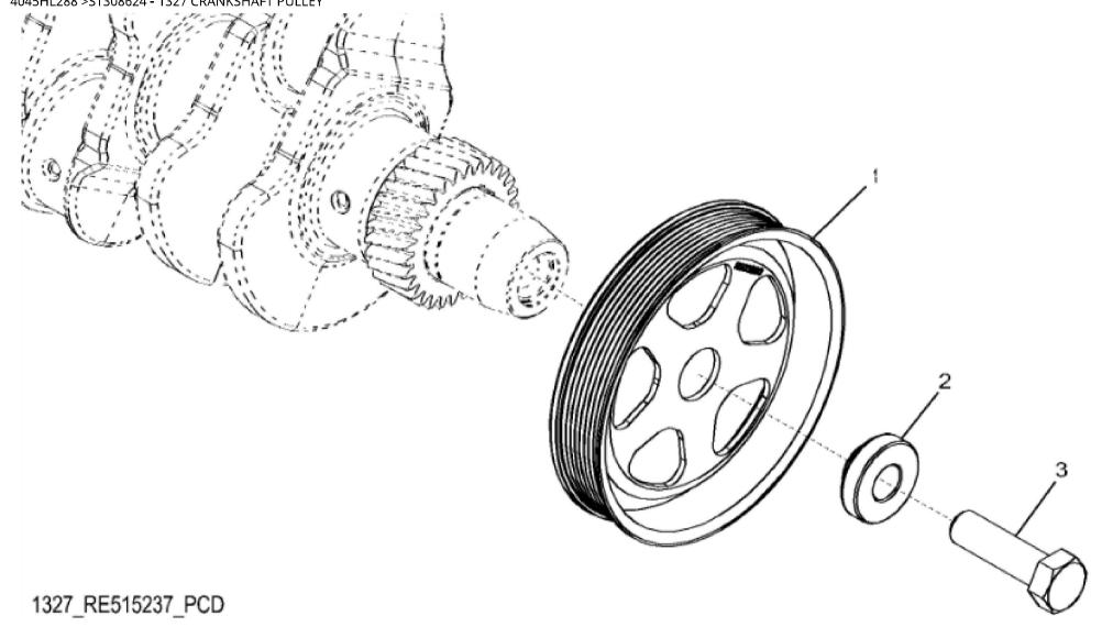
John Deere > Construction And Forestry >BACKHOE, LOADER >410J TMC - BACKHOE, LOADER >410J TMC Backhoe Loader >04A ENGINE 4045HL288-SE503031 >0400A ENGINE 4045HL288-SE503031 4045HL288 >ST308624 - 1327 CRANKSHAFT PULLEY
