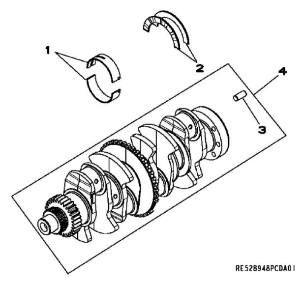
John Deere > Turf And Utility >LOADER, SKID-STEER >4024HT015 - LOADER, SKID-STEER >323D Compact Track Loader >20A ENGINE 4024HT011-RE528665 >ST553 - 4703 (CRANKSHAFT AND BEARINGS)
