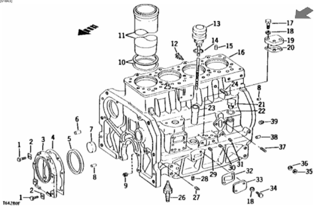
John Deere > Construction And Forestry > BACKHOE, LOADER > 500 - BACKHOE, LOADER > JD500 Series A (-123113) Backhoe Loader > 10 ENGINE > 10-6 - REPLACEMENT CYLINDER BLOCK (DIESEL) [01B03]
