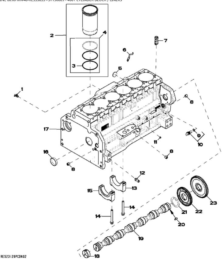
John Deere > Agriculture > TRACTOR > 8295R - TRACTOR > 8295R Tractor (S.N. 001001 - 052200)(6090HRW Engine)(Russian Edition) > 20 ENGINE 6090HRW48-RE533833 > ST130089 - 4601 CYLINDER BLOCK / LINERS
