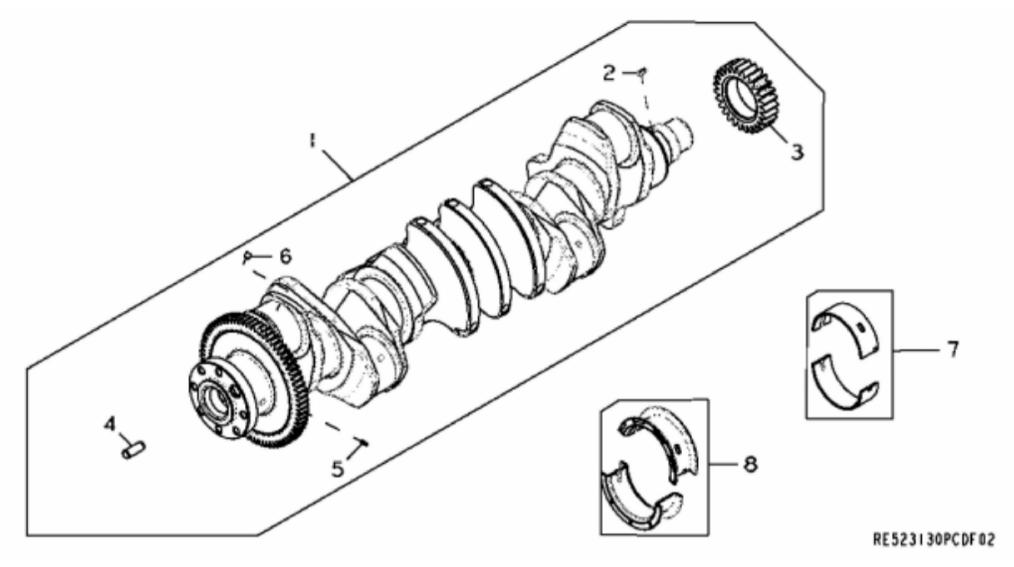
John Deere > Agriculture >TRACTOR >8320R - TRACTOR >8320R Tractor (S.N. 001001 - 052200)(6090HRW Engine)(Russian Edition) >20 ENGINE 6090HRW48-RE533833 >ST130090 - 4701 CRANKSHAFT / BEARINGS
