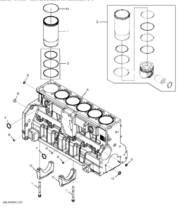
John Deere > Agriculture > TRACTOR > 9430 - TRACTOR > 9430 Tractor (6135HRW Engine)(Russian Edition) > 20 ENGINE 6135HRW02-RE524851 > ST870007 - 4606 CYLINDER BLOCK WITH LINERS (000442 - )
