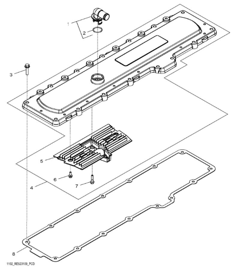
John Deere > Agriculture >TRACTOR >8430T - TRACTOR >8430T Tractor >14 ENGINE 6090HRW04, 6090HRW23-RE522915-RE526800 >ST130073 - 1102 ROCKER ARM COVER
