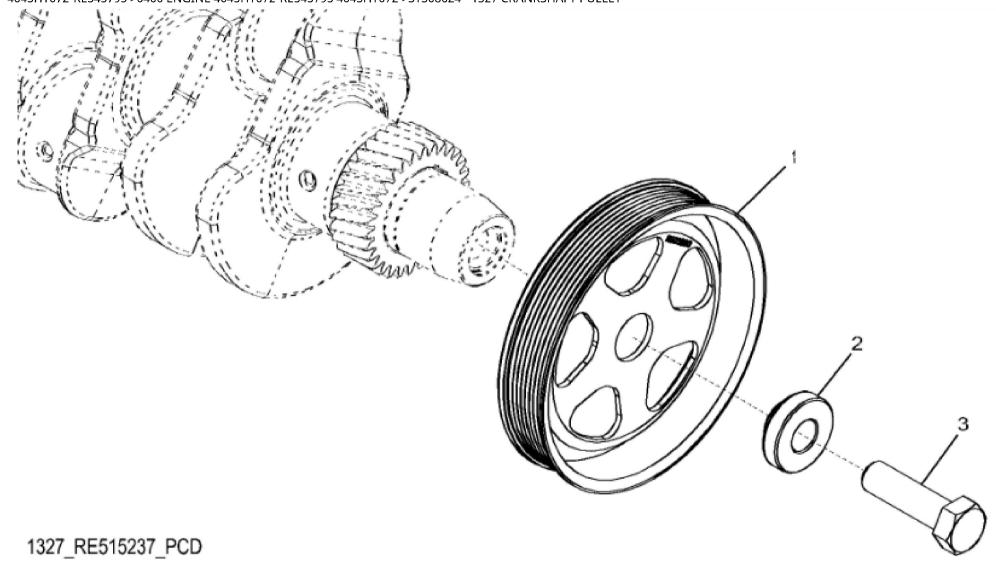
John Deere > Construction And Forestry >BACKHOE, LOADER >310K EP - BACKHOE, LOADER >310K EP Backhoe Loader (Engine 4045HT072)(PIN: 1T0310EK\_\_G219607 - G277403) >04 ENGINE 4045HT072-RE545795 >0400 ENGINE 4045HT072-RE545795 4045HT072 >ST308624 - 1327 CRANKSHAFT PULLEY
