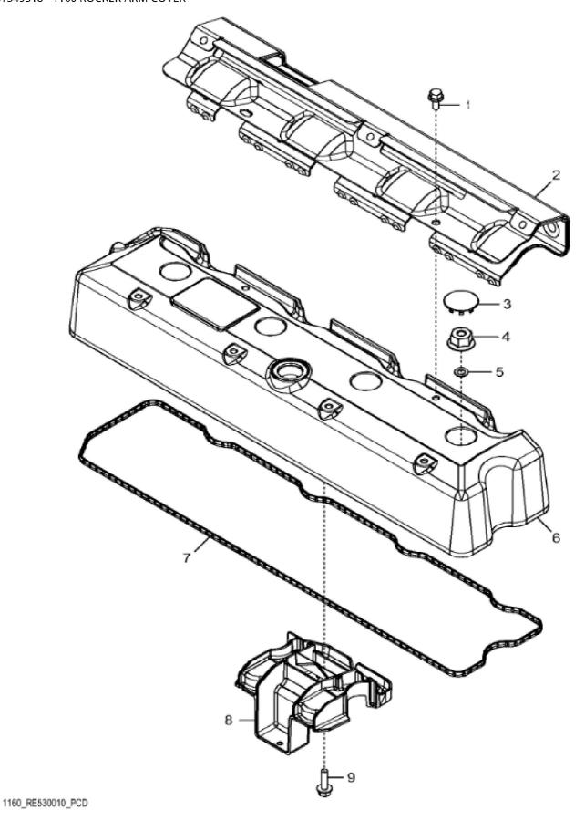
John Deere > Construction And Forestry > BACKHOE, LOADER > 310K EP - BACKHOE, LOADER > 310K EP Backhoe Loader (Engine 4045HT072)(PIN: 1T0310EK\_\_G219607 - G277403) > 04 ENGINE 4045HT072-RE545795 > 0400 ENGINE 4045HT072-RE545795 4045HT072 > ST349518 - 1160 ROCKER ARM COVER
