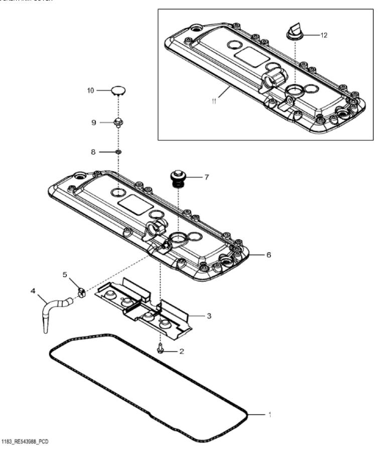
John Deere > Construction And Forestry > BACKHOE, LOADER > 310K - BACKHOE, LOADER > 310K Backhoe Loader (Engine 4045HT073)(PIN: 1T0310KX\_\_E219607 - E277404) > 04 ENGINE 4045HT073-RE546630 > 0400 ENGINE 4045HT073-RE546630 4045HT073 > ST400926 - 1183 ROCKER ARM COVER
