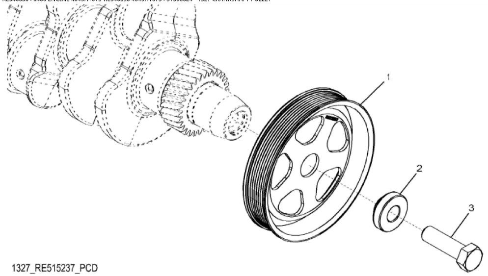
John Deere > Construction And Forestry > BACKHOE, LOADER > 310K - BACKHOE, LOADER > 310K Backhoe Loader (Engine 4045HT073)(PIN: 1T0310KX\_\_E219607 - E277404) > 04 ENGINE 4045HT073-RE546630 > 0400 ENGINE 4045HT073-RE546630 4045HT073 > ST308624 - 1327 CRANKSHAFT PULLEY
