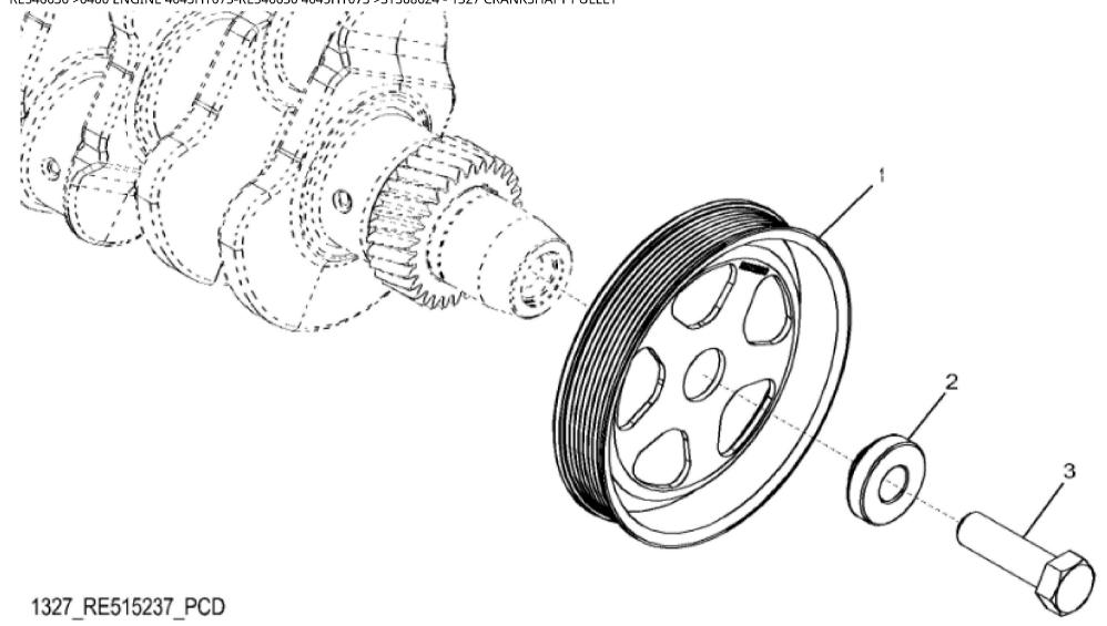
John Deere > Construction And Forestry > BACKHOE, LOADER > 310SK - BACKHOE, LOADER > 310SK Backhoe Loader (Engine 4045HT073)(PIN: 1T0310SK\_\_E219607 - E277407) > 04 ENGINE 4045HT073-RE546630 > 0400 ENGINE 4045HT073-RE546630 4045HT073 > ST308624 - 1327 CRANKSHAFT PULLEY
