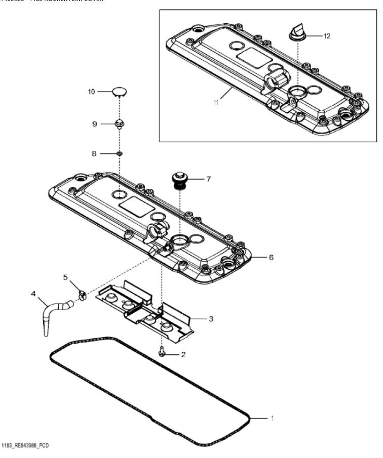
John Deere > Construction And Forestry > BACKHOE, LOADER > 310SK - BACKHOE, LOADER > 310SK Backhoe Loader (Engine 4045HT073)(PIN: 1T0310SK\_\_E219607 - E277407) > 04 ENGINE 4045HT073-RE546630 > 0400 ENGINE 4045HT073-RE546630 4045HT073 > ST400926 - 1183 ROCKER ARM COVER
