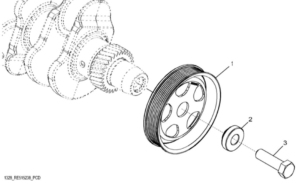
John Deere > Construction And Forestry >BACKHOE, LOADER >310SK - BACKHOE, LOADER >310SK Backhoe Loader (Engine 4045HT054,4045HT085,4045HT086,4045TT096)(PIN: 1T0310SK\_ C219607 - C277407)(PIN: 1T0310SK\_ D219607 - D277407) >04A ENGINE 4045HT086-RE566132 >0400A ENGINE 4045HT086-RE566132 4045HT086 >ST628039 - 1328 CRANKSHAFT PULLEY
