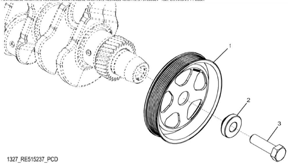
John Deere > Construction And Forestry > BACKHOE, LOADER > 310SK TC - BACKHOE, LOADER > 310SK TC (TMC) Backhoe Loader (Engine 4045HT063,4045HT073)(PIN: 1T0310TK\_\_E219607 - E270402) > 044 ENGINE 4045HT073-RE546630 > 0400A ENGINE 4045HT073-RE546630 4045HT073 > ST308624 - 1327 CRANKSHAFT PULLEY
