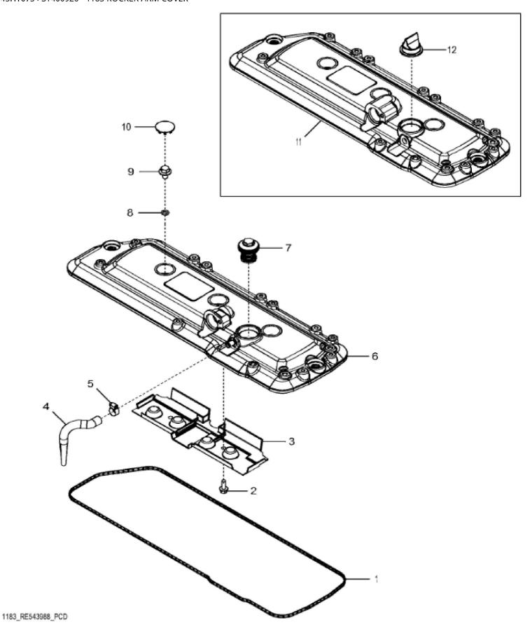
John Deere > Construction And Forestry > BACKHOE, LOADER > 310SK TC - BACKHOE, LOADER > 310SK TC (TMC) Backhoe Loader (Engine 4045HT063,4045HT073)(PIN: 1T0310TK\_\_E219607 - E270402) > 044 ENGINE 4045HT073-RE546630 > 0400A ENGINE 4045HT073-RE546630 4045HT073 > ST400926 - 1183 ROCKER ARM COVER
