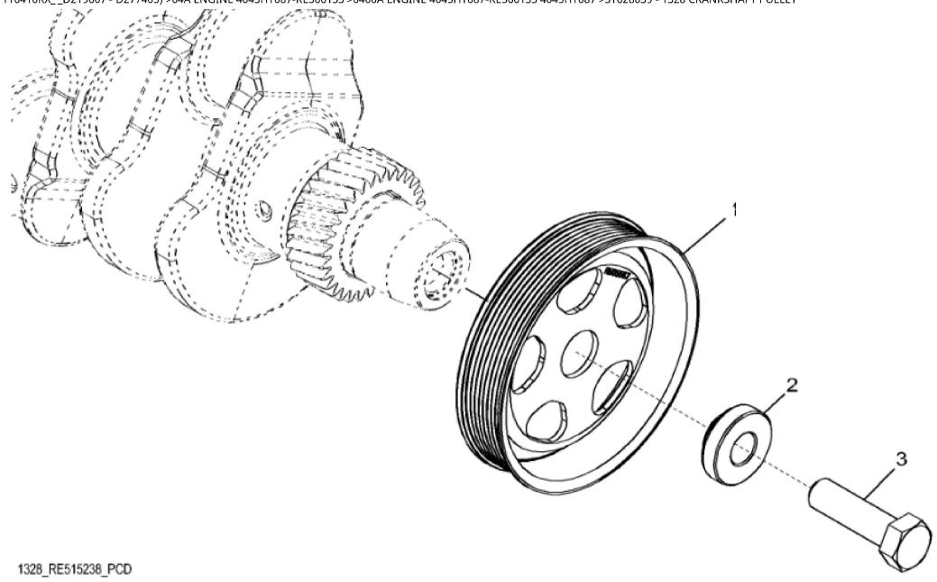
John Deere > Construction And Forestry > BACKHOE, LOADER > 410K - BACKHOE, LOADER > 410K Backhoe Loader (Engine 4045HT054,4045HT087,4045TT096)(PIN: 1T0410KX\_\_C219607 - C277405)(PIN: 1T0410KX\_\_D219607 - D277405) > 04A ENGINE 4045HT087-RE566133 > 0400A ENGINE 4045HT087-RE566133 4045HT087 > ST628039 - 1328 CRANKSHAFT PULLEY
