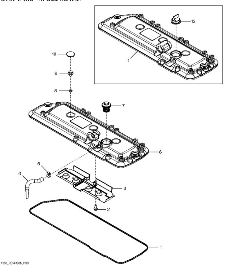
John Deere > Construction And Forestry > BACKHOE, LOADER > 410K TC - BACKHOE, LOADER > 410K TC (TMC) Backhoe Loader (Engine 4045HT063, 4045HT073)(PIN: 1T0410TK\_\_E219607 - E268557) > 044 ENGINE 4045HT073-RE546630 > 0400A ENGINE 4045HT073-RE546630 4045HT073 > ST400926 - 1183 ROCKER ARM COVER
