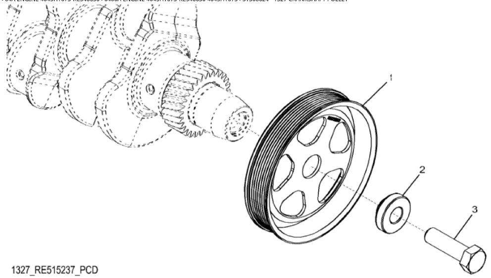
John Deere > Construction And Forestry > BACKHOE, LOADER > 410K TC - BACKHOE, LOADER > 410K TC (TMC) Backhoe Loader (Engine 4045HT063, 4045HT073)(PIN: 1T0410TK\_\_E219607 - E268557) > 044 ENGINE 4045HT073-RE546630 > 0400A ENGINE 4045HT073-RE546630 4045HT073 > ST308624 - 1327 CRANKSHAFT PULLEY
