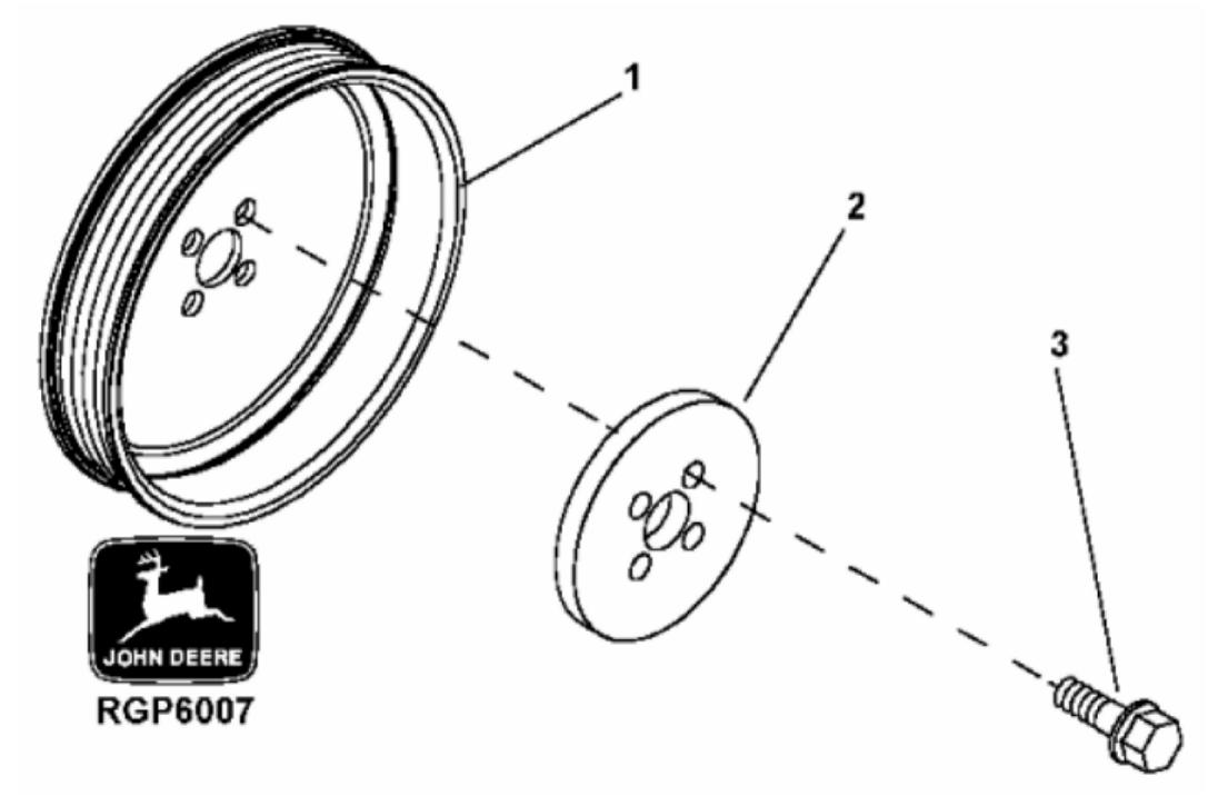
John Deere > Construction And Forestry >BACKHOE, LOADER >310K - BACKHOE, LOADER >310K Backhoe Loader (Engine 4045TT096, 4045TBZ01)(PIN: 1BZ310KX\_ C000001- ) >04A ENGINE 4045TBZ01-RE564738 >0400A ENGINE 4045TBZ01-RE564738 4045TBZ01 >ST587568 - 1302 CRANKSHAFT PULLEY
