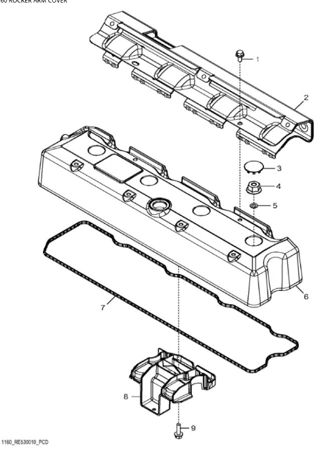
John Deere > Construction And Forestry >BACKHOE, LOADER >310L EP - BACKHOE, LOADER >310L EP Backhoe Loader (Engine 4045HT072)(PIN: 1T0310EL\_\_G273920- ) >04 ENGINE 4045HT072-RE545795 >0400 ENGINE 4045HT072-RE545795 4045HT072 >ST349518 - 1160 ROCKER ARM COVER
