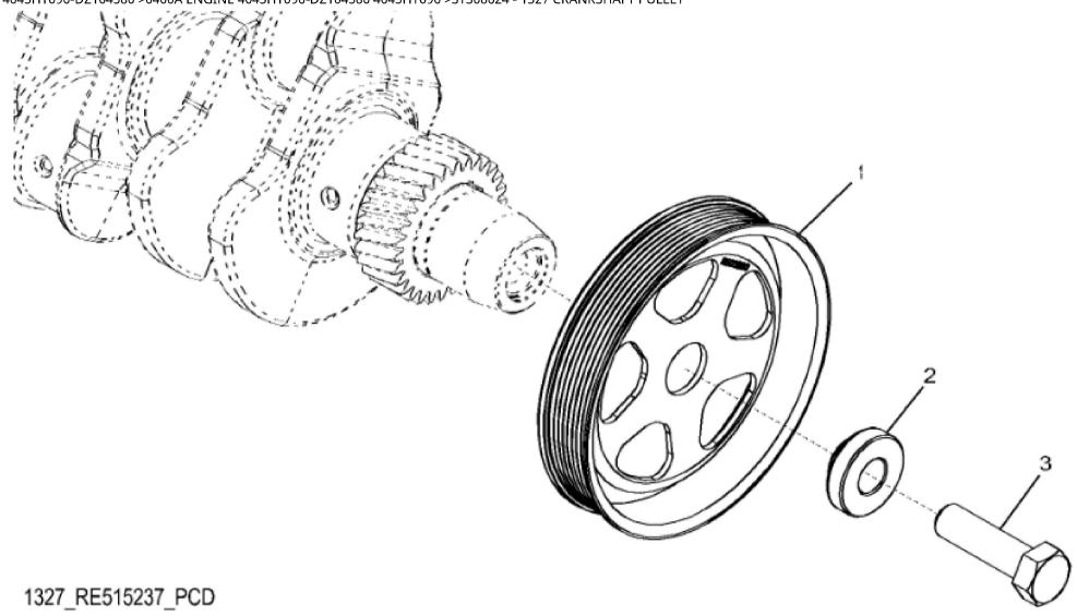
John Deere > Construction And Forestry > BACKHOE, LOADER > 310L - BACKHOE, LOADER > 310L Backhoe Loader (Engine 4045HT082,4045HT096)(PIN: 1T0310LX\_\_F273920- ) > 04A ENGINE 4045HT096-DZ104580 > 0400A ENGINE 4045HT096-DZ104580 4045HT096 > ST308624 - 1327 CRANKSHAFT PULLEY
