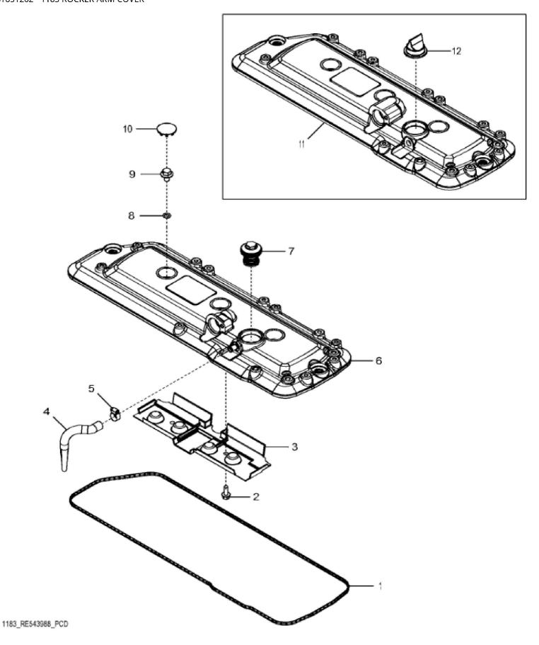
John Deere > Construction And Forestry > BACKHOE, LOADER > 310L - BACKHOE, LOADER > 310L Backhoe Loader (Engine 4045HT082,4045HT096)(PIN: 1T0310LX\_\_F273920- ) > 04A ENGINE 4045HT096-DZ104580 > 0400A ENGINE 4045HT096-DZ104580 4045HT096 > ST851262 - 1183 ROCKER ARM COVER
