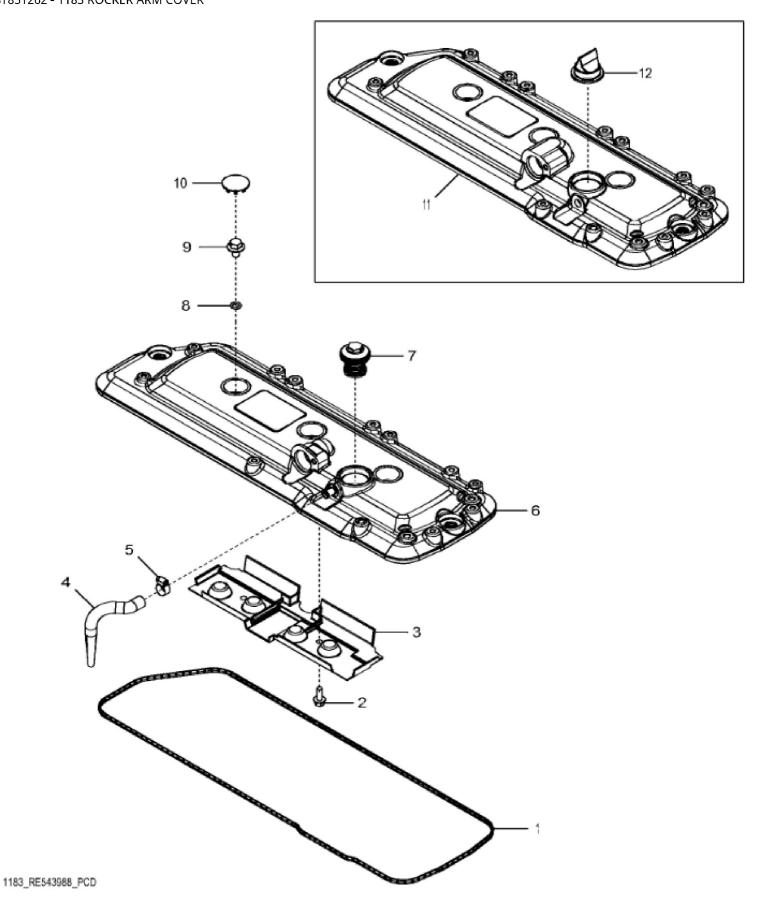
John Deere > Construction And Forestry > BACKHOE, LOADER > 310SL - BACKHOE, LOADER > 310SL Backhoe Loader (Engine 4045HT082,4045HT096)(PIN: 1T0310SL\_\_F273920- ) > 04A ENGINE 4045HT096-DZ104580 > 0400A ENGINE 4045HT096-DZ104580 4045HT096 > ST851262 - 1183 ROCKER ARM COVER
