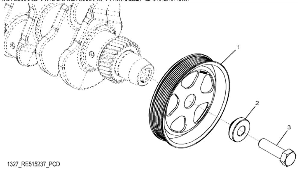
John Deere > Construction And Forestry >BACKHOE, LOADER >310SL - BACKHOE, LOADER >310SL Backhoe Loader (Engine 4045HT082,4045HT096)(PIN: 1T0310SL\_\_F273920- ) >04A ENGINE 4045HT096-DZ104580 >0400A ENGINE 4045HT096-DZ104580 4045HT096 >ST308624 - 1327 CRANKSHAFT PULLEY
