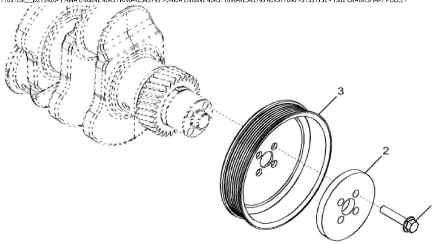
John Deere > Construction And Forestry >BACKHOE, LOADER >310SL - BACKHOE, LOADER >310SL Backhoe Loader (Engine 4045HT085, 4045HT086, 4045TT096)(PIN: 1T0310SL\_\_C273920-)(PIN: 1T0310SL\_\_D273920-) > 044 ENGINE 4045TT096-RE545793 > 0400A ENGINE 4045TT096-RE545793 4045TT096 > ST351152 - 1302 CRANKSHAFT PULLEY
