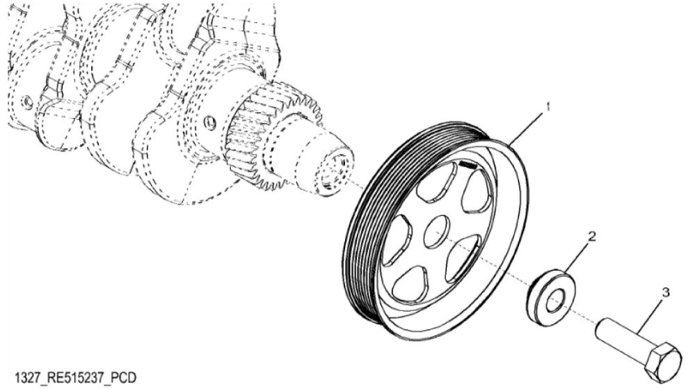
John Deere > Construction And Forestry >BACKHOE, LOADER >315SL - BACKHOE, LOADER >315SL Backhoe Loader (Engine 4045HT082,4045HT096)(PIN: 1T0315SL\_F273920-) >04A ENGINE 4045HT096-DZ104580 >0400A ENGINE 4045HT096-DZ104580 4045HT096 >ST308624 - 1327 CRANKSHAFT PULLEY
