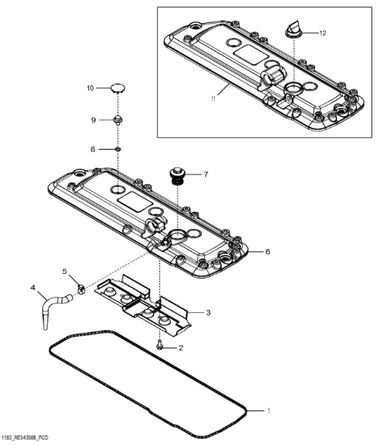
John Deere > Construction And Forestry >BACKHOE, LOADER >315SL - BACKHOE, LOADER >315SL Backhoe Loader (Engine 4045HT082,4045HT096)(PIN: 1T0315SL\_F273920-) >04A ENGINE 4045HT096-DZ104580 >0400A ENGINE 4045HT096-DZ104580 4045HT096 >ST851262 - 1183 ROCKER ARM COVER
